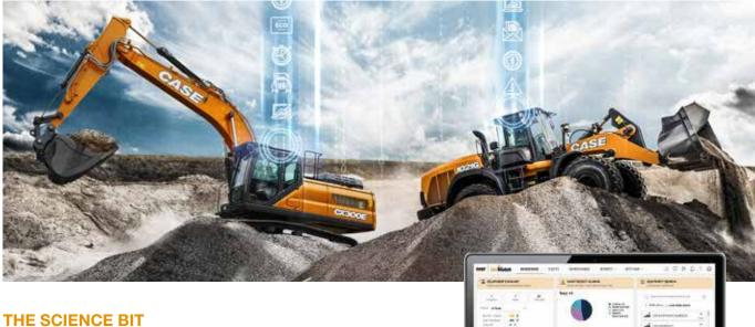
The CASE SiteWatch telematics system uses a high-tech control unit mounted on each machine to collate information from that machine and from GPS satellites. This data is then sent wirelessly through the mobile communication networks to the CASE Telematics Web Portal.
