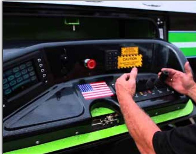
*Configuration and control of your PTO functions has never been easier. User defined presets allow the engine and PTO to be set for optimal operation under any load. PTO controls are in the cab and can also be located remotely on the body and can operate up to two PTO's.*
