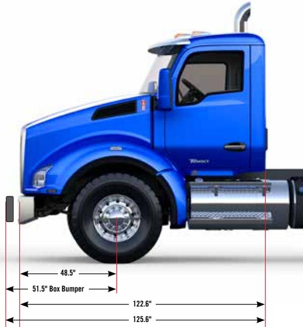
The T880 is one of the most proven and versatile work trucks ever conceived. Its "standard" set-back front axle configuration offers the perfect foundation for a myriad of tough-duty solutions requiring superior strength, reliability and operating efficiency.
