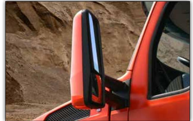
*Durable aerodynamic side mirrors are cowl mounted for better stability and located farther forward and lower to optimize rearward visibility. The convex portion is 37 percent larger than Kenworth's standard convex mirror design.*
