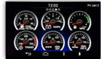
*Pre-loaded virtual gauges include oil temperature, transmission temperature, manifold boost, present and average fuel economy, DPF status and engine torque.*
