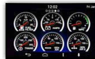
*Pre-loaded virtual gauges include oil temperature, transmission temperature, manifold boost, present and average fuel economy, DPF status and engine torque.*
