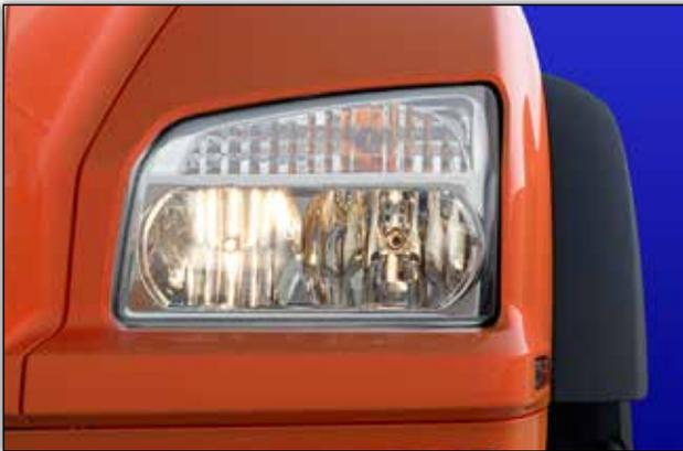
*Complex reflector halogen headlights offer the lighting performance of projector beam systems without the extra cost. Designed with extra thick polycarbonate lens and UV inhibitor, the headlamps will stand up to years of service without any complaints.*
