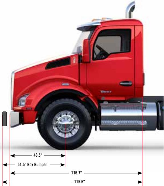
This highly maneuverable set-back front axle model has been designed for maximum productivity, optimized weight distribution and body-mounting flexibility in applications that call for a lightweight yet robust solution.
