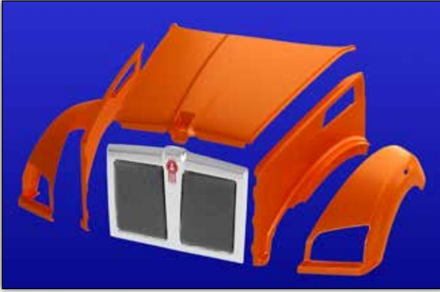
*The 5-piece T880 hood offers bolt-on fenders for quick replacement to get you back on the work site. Each fender can be replaced in less than two hours.*
